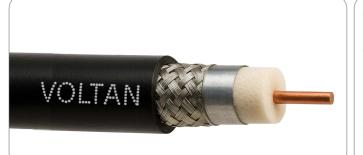
Voltan RG 11U is a common type of coaxial cable in a wide variety of residential and commercial applications. This RG 11 type cables have become the standard for CATV/MATV, Broadband, HDTV and Satellite Broadcasting Transmission use, has a copper-coated steel center conductor and a combination aluminum foil/aluminum braid shield, with coverage about 95% and PVC/LSZH Outer jacket.
