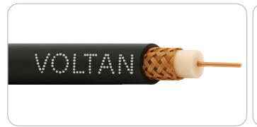
Voltan RG 6U type cables are also used in professional video applications, carrying either baseband analog video signals in closed circuit television (CCTV) or serial digital interface (SDI) signals; in these applications, the center conductor is ordinarily solid copper, the shielding is much heavier (90% copper braid), and tolerances are more tightly controlled, to improve impedance stability. RG6 can be used as a branch cable with Standard Transmission distance up to 450m.
