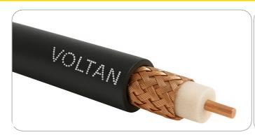
Voltan RG 11U type cables are also used in professional video applications, carrying either baseband analog video signals in closed circuit television (CCTV) or serial digital interface (SDI) signals. in these applications, the center conductor is ordinarily solid copper, the shielding is much heavier (90% Bare copper braid), and tolerances are more tightly controlled, to improve impedance stability. RG11 can be used as a trunk cable with standard Transmission distance up to 600m
