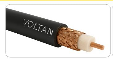
Voltan RG 11U type cables are also used in professional video applications, carrying either baseband analog video in closed-circuit television (CCTV) signals or serial digital interface (SDI) signalsp; in these applications, the center conductor is ordinarily solid copper, the shielding is such heavier (60% Bare copper braid), and tolerances are more tightly controlled, to improve impedance stability. RG 11 can be used as a trunk cable with standard Transmission distance up to 600m.
