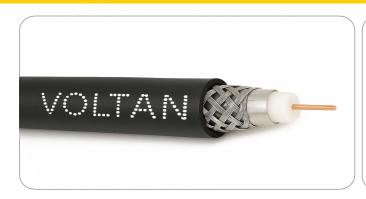
Voltan RG 6U is a common type of coaxial cable used in a wide variety of residential and commercial applications. This RG 6 type cables have become the standard for CATV, has a copper-coated steel center conductor and a combination aluminum foil/aluminum braid shields, typically with low coverage about 60%. RG6 can be used as a branch cable with Standard Transmission distance up to 450m.Outer jacket is made up of UV Protective PE jacket.
