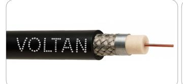
Voltan RG 6U is a common type of coaxial cable used in a wide variety of residential and commercial applications. This RG 6U type cables have become the standard for CATV, has a copper-coated steel center conductor and a combination aluminium foil/ aluminium braid shield, typically with high coverage about 90%. RG 6U can be used as a branch cable with standard transmission distance up to 450m.
