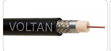
Voltan RG 6U is a common type of coaxial cable used in a wide variety of residential and commercial applications. This RG 6U type cables have become the standard for CATV, has a copper-coated steel center conductor and a combination aluminium foil/ aluminium braid shield, typically with low coverage about 60%. RG 6U can be used as a branch cable with standard transmission distance up to 450m.
