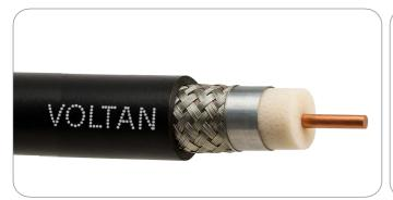
Voltan RG 11U is a common type of coaxial cable in a wide variety of residential and commercial applications. This RG 11 type cables have become the standard for CATV/MATV, Broadband, HDTV and Satellite Broadcasting Transmission use, has a copper-coated steel center conductor and a combination aluminium foil/aluminium braid shield, typically with low coverage about 60%. RG11 can be used as a trunk cable with standard Transmission distance up to 600m.
